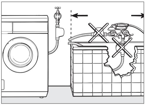
The plastic casing of the water connection contains an electric component. The Waterproof system must only be connected to its own stopcock. It must not be connected to mixer taps or similar and must not be fitted in areas where there is the risk of water or other liquids reaching it.
